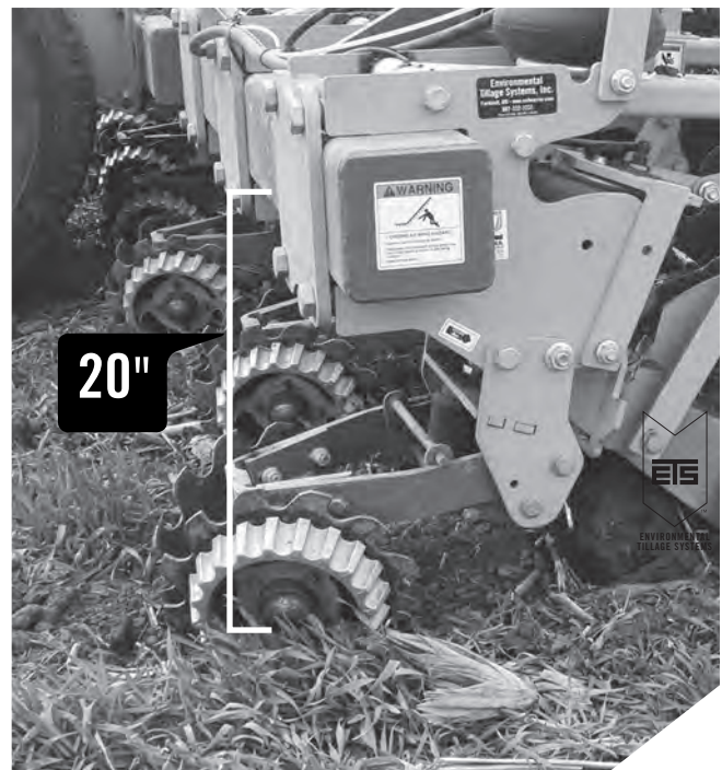
Distance between the bottom of the toolbar and ground
