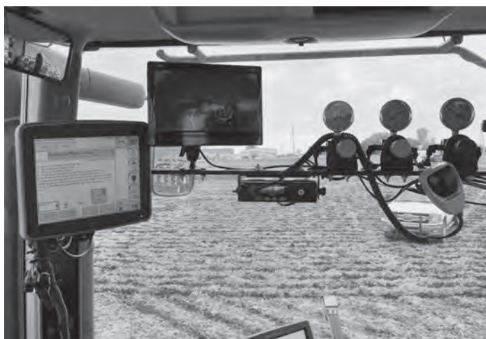
Typical installation of regulators and switch boxes.
