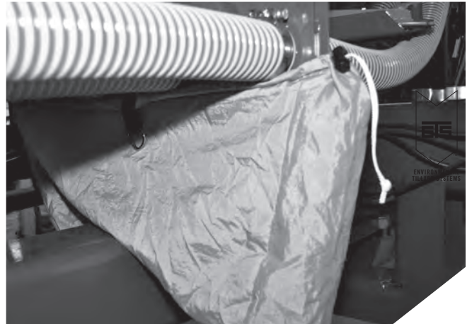
Meter calibration bag attached to collector bottom
