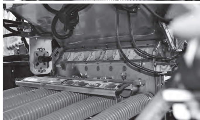
TOP: Meter roll with access door attached BOTTOM: Meter roll rear access door removed
