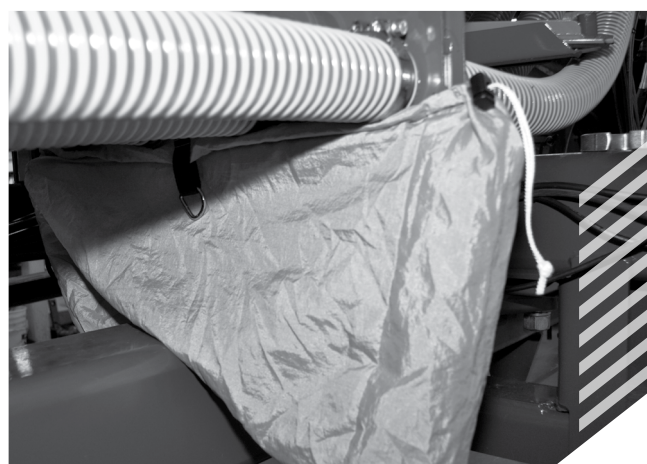
Meter calibration bag attached to collector bottom
