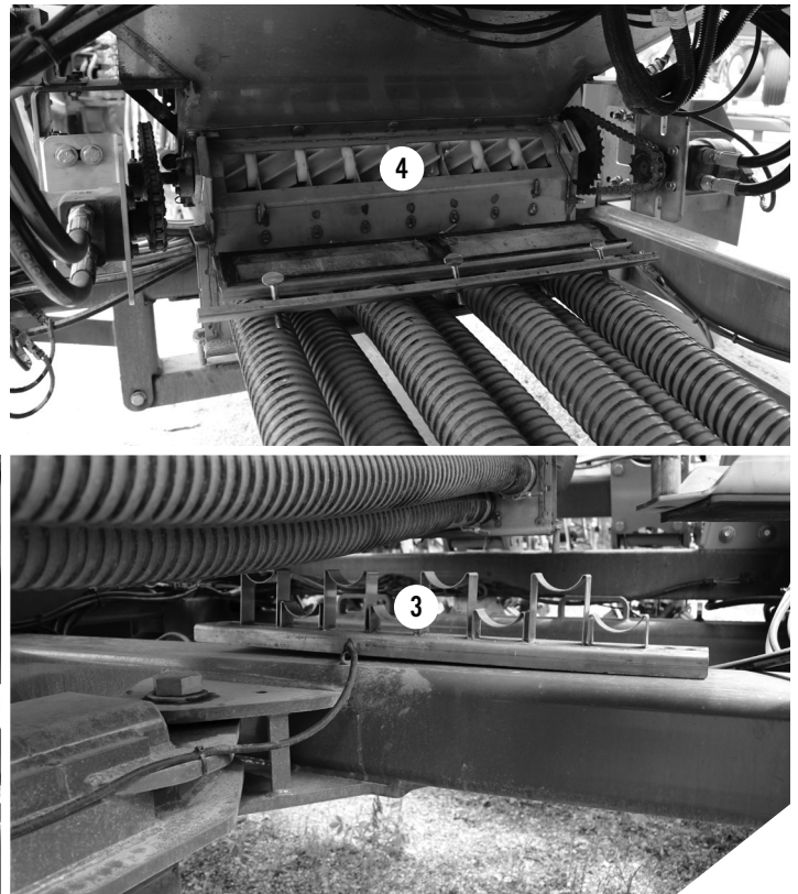
TOP: Meter roll with rear access door removed BOTTOM: Meter roll collector bottom insert
